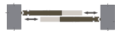
2 ante scorrevoli parallele, binario ad incasso 2 vie Double parallel sliding door with double way hidden ceiling rail
