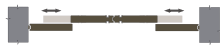
4 ante parallele scorrevoli a soffitto, binario 2 vie Quadruple parallel sliding door, 2 ways ceiling-rail
