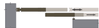
2 ante scorrevoli a trascinamento, binario ad incasso 2 vie Double parallel sliding door with link and drag system, double way hidden ceiling rail
