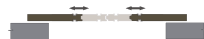
2 ante scorrevoli, binario ad incasso 1 via Double sliding door with one way hidden ceiling rail
